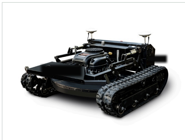
T1-900A — tracked hybrid-electric autonomous mower
